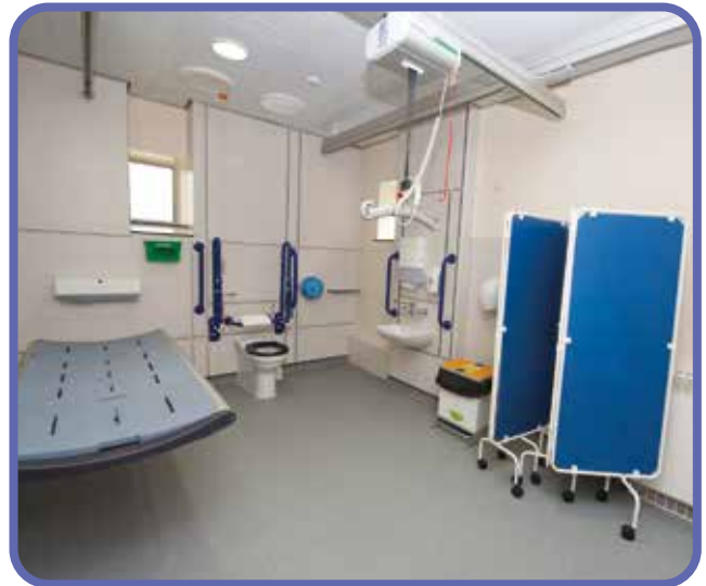
Changing Places facility for assisted use: minimum 3m by 4m in size, including a centrally located WC with space for assistants either side, adult-sized height-adjustable changing bench, a ceiling track hoist and privacy screen
